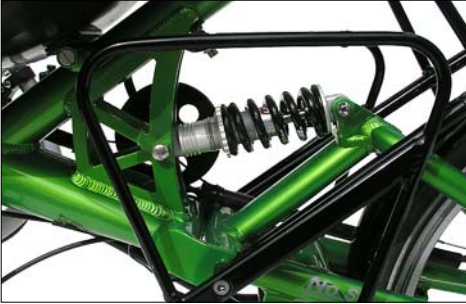
Steel spring suspension element with fixed damping rate.
