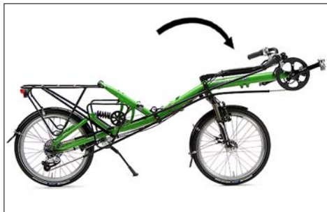
Bring right pedal to the front and fold handlebars forward
