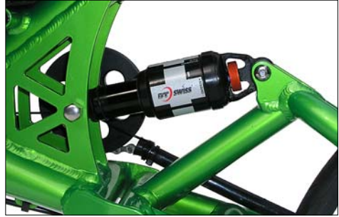
Air Shock DT-Swiss XM180. Damping is adjusted with the red knob at the rear end.
