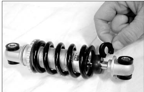
The suspension travel is adjusted by adding clips to the piston rod of the spring element.
