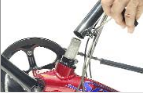
After you have undone the clamping screw of the stem you can take off the stem.
