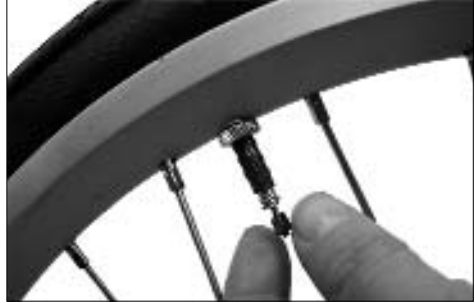
Before pumping up the tire, you have to undo the little knurled nut on the valve.
