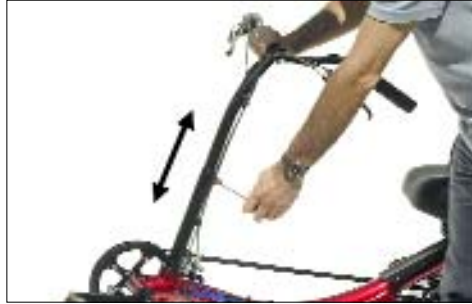
You can adjust the height of the handlebars by undoing the clamping screw.
