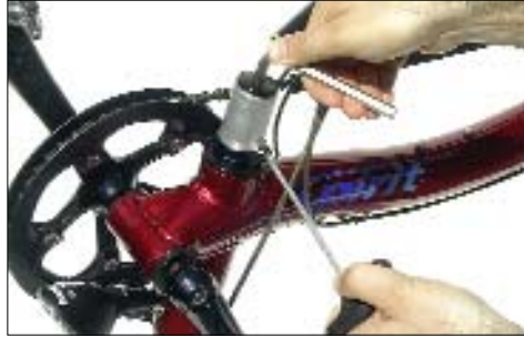
Adjusting the headset with mounted adjustment bushing.
