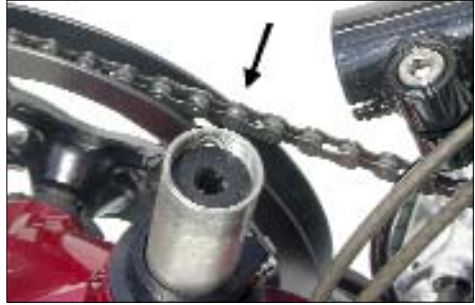
In the inner fork steerer tube there is the adjustment screw for the pre-load.
